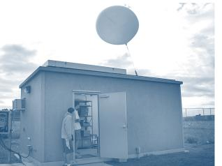
**RADIOSONDE** A radiosonde is a balloon-borne instrument platform with radio transmitting capabilities. Like driftsondes, radiosondes carry pressure, temperature, and humidity instrumentation. These sensors gather and send back data about atmospheric conditions during an upward
