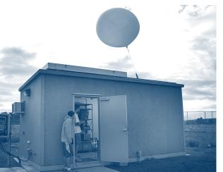
**RADIOSONDE** A radiosonde is a balloon-borne instrument platform with radio transmitting capabilities. Like driftsondes, radiosondes carry pressure, temperature, and humidity instrumentation. These sensors gather and send back data about atmospheric conditions during an upward
